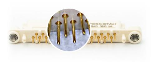
The angle of the socket wires allows tight control of the Pin insertion and extraction forces. The spring wires are smoothly defected to make line contact with the Pin. The rugged connector with special buffer structure between
